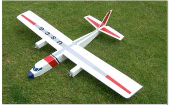
Ted Remmer's Aerovan twin from a magazine plan sports two cheap brushless motors on a 3900 2S LiPo and flies extremely well
