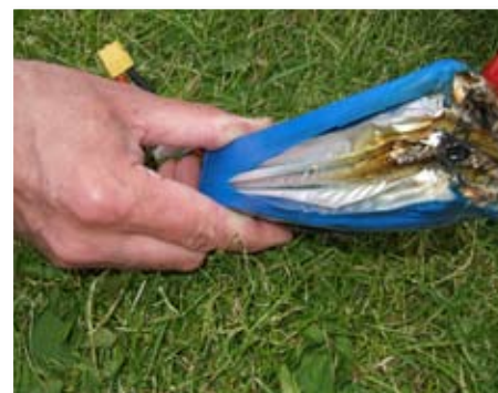
A reminder that 5000 mAh LiPos don't fare well in crashes – lots of smoke but no fire, luckily. The battery hit the back of the motor in the crash
