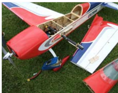
Barry Hurst's large E-flite Extra – damage was more or less limited to the loss of the wing and is repairable. The model runs a Turnigy G45 motor and 70 A ESC on 4S LiPos
