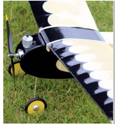
Not that you'd know it! This is Mike Cawood's nose-weight in the form of a 'diesel motor' made from laminated 1p and 2p coins! Top job!
