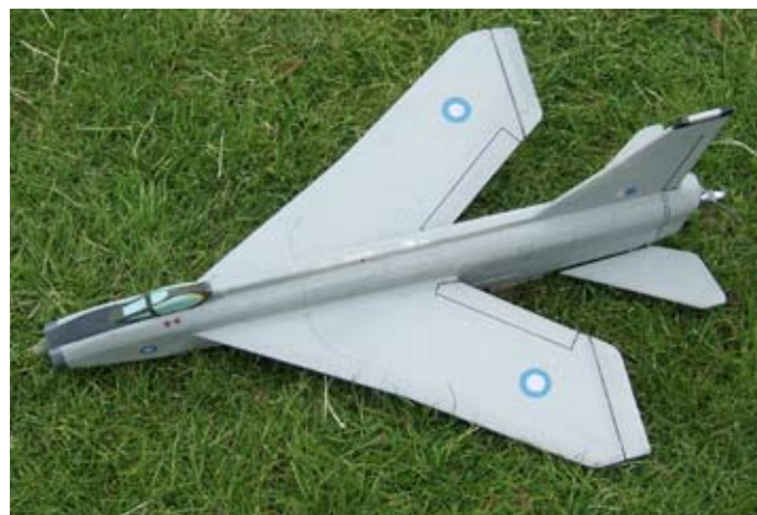
Tony Oliver's Lightning also runs a rewind 10 g outrunner, 10 A ESC and 800 mAh 2S LiPos, as does his Javelin
